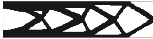
Fig. 2 Optimized topology for 60 kN with the open filter
