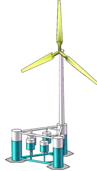
Fig. 2. Hybrid system of a floating wind platform and multiple heaving WECs.
