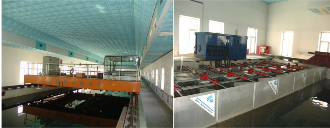
Fig. 12. Wave tank, trailer, and wave maker at Harbin Engineering University.
