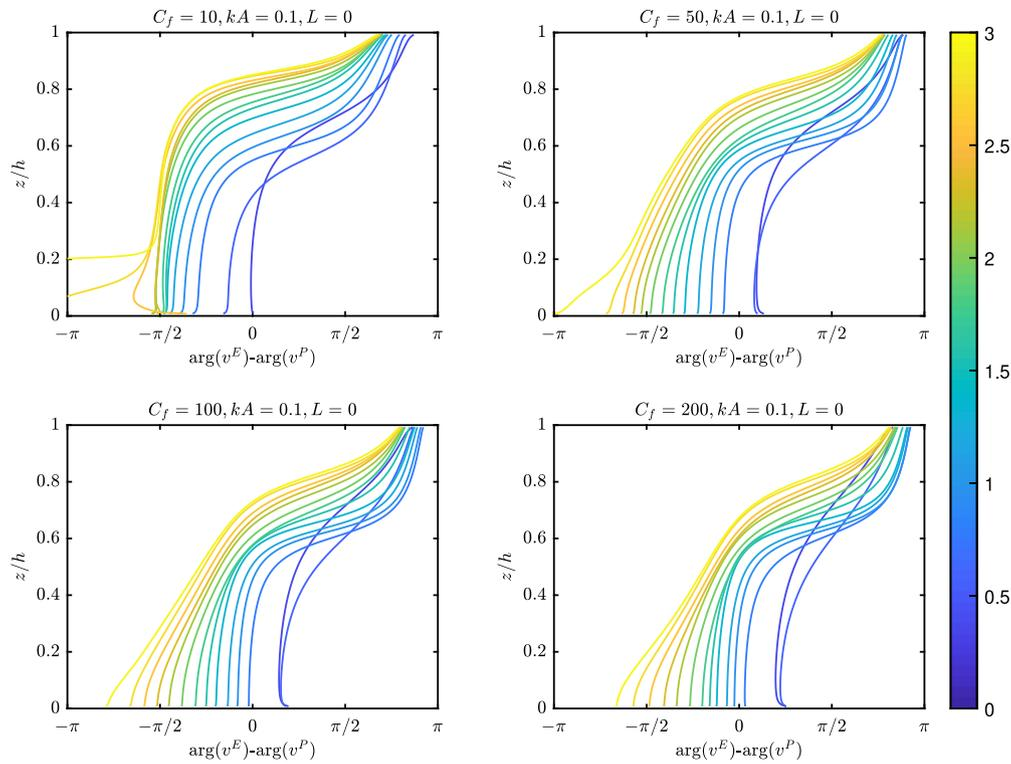
**Fig. 10.** Phase of velocity through the porous wall due to evanescent components of the wave field relative to phase of progressive components, for  $kA = 0.1$ ,  $C_f = 10, 50, 100, 200$  and  $L = 0$ . Colour of line indicates value of  $kh$ . (For interpretation of the references to colour in this figure legend, the reader is referred to the web version of this article.)
