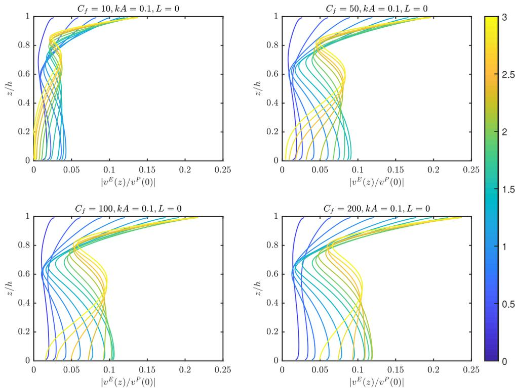
Fig. 9. Relative magnitude of velocity through the porous wall due to evanescent components of the wave field against depth for  $kA = 0.1$ ,  $C_f = 10, 50, 100, 200$  and  $L = 0$ . Colour of line indicates value of  $kh$ . (For interpretation of the references to colour in this figure legend, the reader is referred to the web version of this article.)
