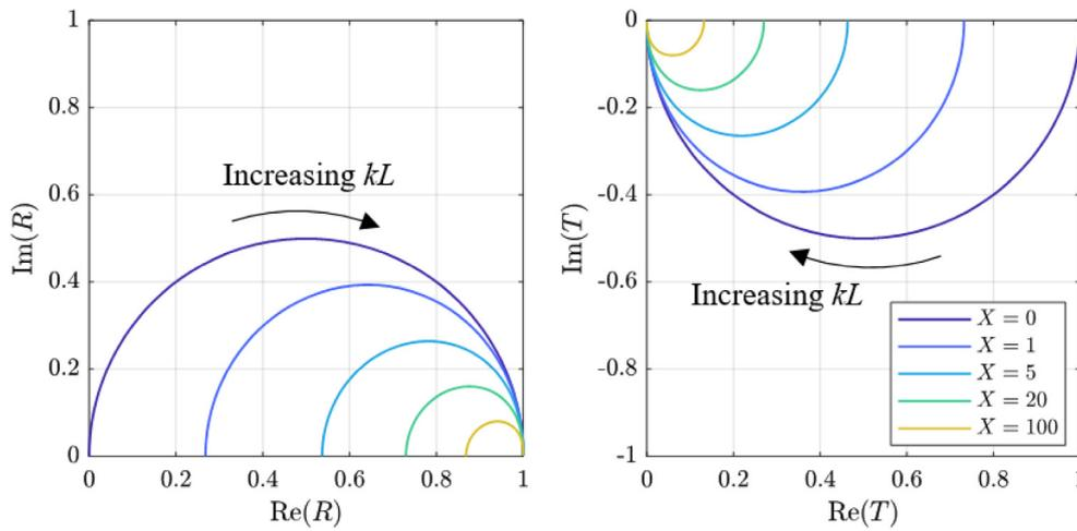
Fig. 6. Real and imaginary parts of  $R$  and  $T$  for fixed values of  $X$  and  $0 \leq kL < \infty$ . (For interpretation of the references to colour in this figure legend, the reader is referred to the web version of this article.)
